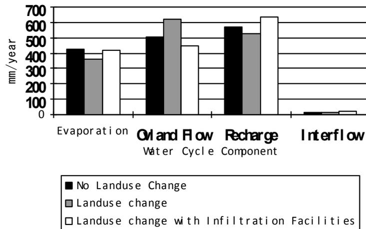
Fig. 6 Main water balance components affected by land use change and recovery measures.
