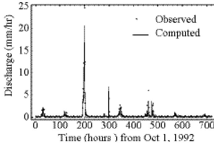
Fig. 4 Comparison of observed and computed discharge for the year 1992.
