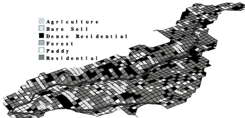
Fig. 2 Maehara sub-catchment with landuse distribution (grid size 50 m × 50 m).
